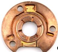
The tolerances inside a turbocharger is absolutely finite. Contaminated or dirty oil will scratch / score the bearings and lead to rapid wear and the turbocharger will fail ultimately.
